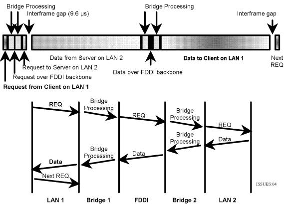
Figure 4: Timing relationships for a high-speed backbone bridged or routed architecture.
