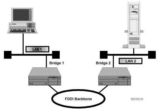
Figure 3: Bridged network architecture using a high-speed backbone network.
