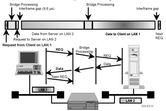
Figure 2: Impact of inserting a bridge on "ping-pong" protocol performance.
